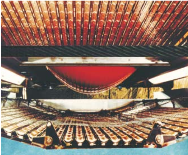
Figure 7: Thermoforming plant for boat hulls
