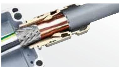
**Progress® EMC cable glands** made of brass ensure a low-impedance connection between the braided shield and the metal chassis while maintaining secure cable routing.
