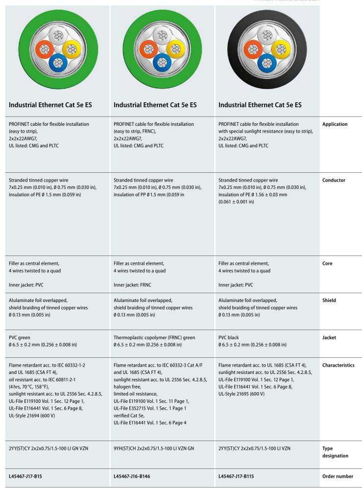
PE = Polyethylene PVC = Polyvinylchloride LEONI 13
