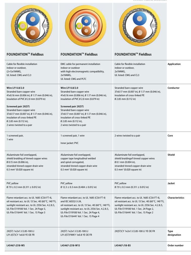
PE = Polyethylene PVC = Polyvinylchloride LEONI 35
