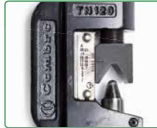
Professional manual mechanical tool suitable for crimping A-M Cu lugs and non-insulated L-M and L-P connectors.
