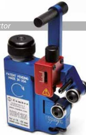
HB12N cable stripping tool removes the semiconductor layer by being manually rotated around the cable while lateral advancement is achieved automatically. Safe and convenient, it can be used on cables with a semi-con diameter between 18 - 60 mm.
