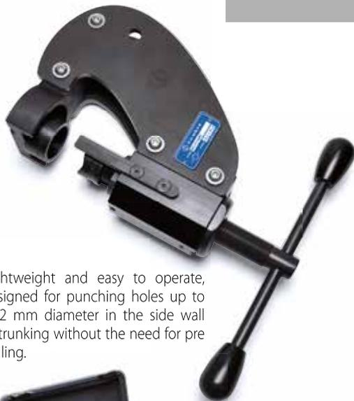
Lightweight and easy to operate, designed for punching holes up to 47,2 mm diameter in the side wall of trunking without the need for pre drilling.
