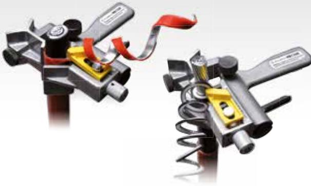
Universal cable stripping tool for external sleeves of Low/Medium Voltage cables  $\varnothing$  12,7 to 63,5 mm and primary insulator in XLPE max  $\varnothing$  38,1 mm
