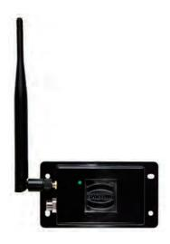
It processes the readings from the accelerometer probe and wirelessly sends them to the host computer
