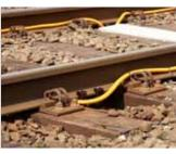
**PMAFIX and PMAFLEX** in wheel sensor applications
