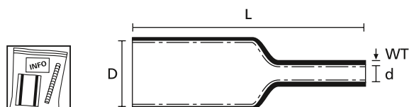
Heat Shrinkable Tubing 4:1 with adhesive
