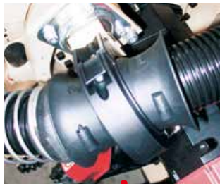
— Tube clamp with ball joint sleeve
