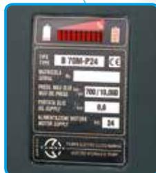
Battery residual power level display
